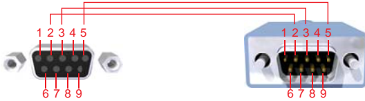
Only Pins 2 (RX), 3 (TX), and 5 (Ground) are used on the RS-232 serial interface
